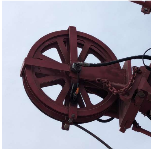
Figure 13 Wireline RPM Sensor Assembly on bottom right of picture
