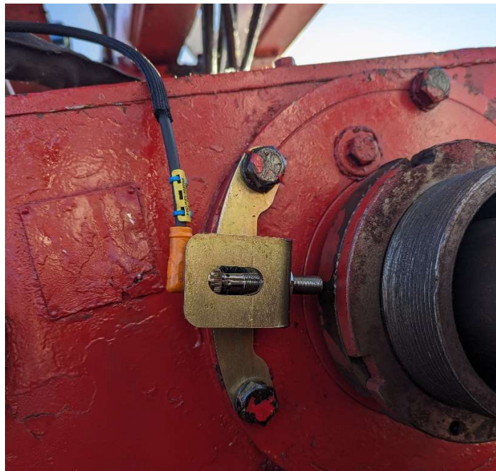
Figure 10 Head speed mounted on supplied bracket after being mounted.
