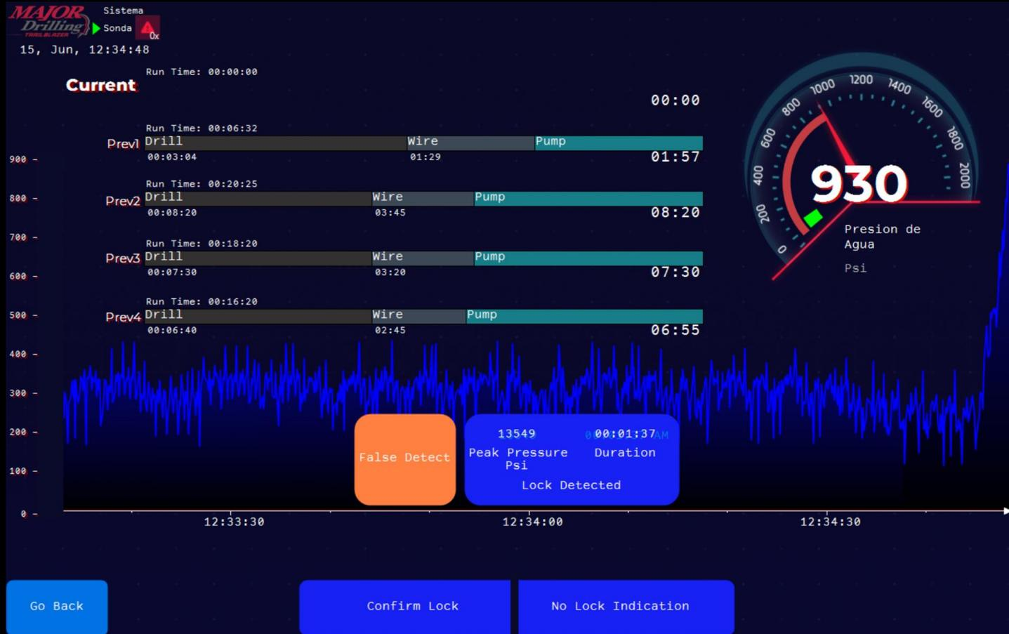
the real-time Pump Pressure enhanced Display.
