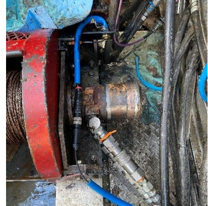
Figure 20, 21, 22, Wireline RPM Bracket, cut out Flag on Drum, Cable Disconnect
