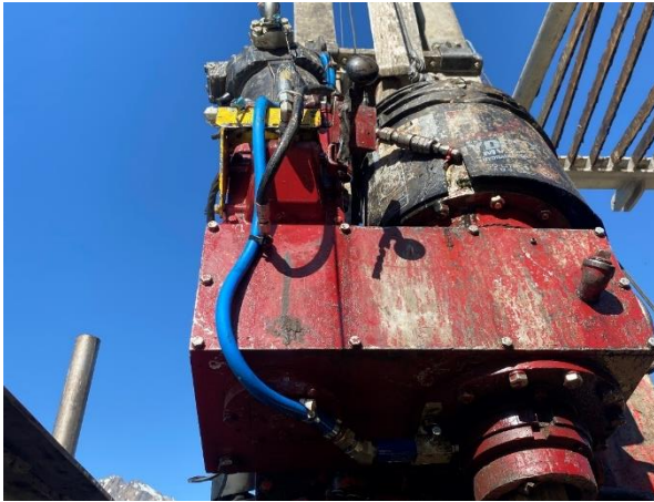
Figure 18, 19 Installation of Sensor, Cable Disconnect Location with Hydraulic Disconnect.
