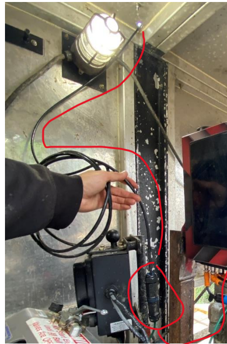
Figure 32, 33, Hole for Starlink Cable to Run through, Starlink Disconnect to Rock5 Unit
