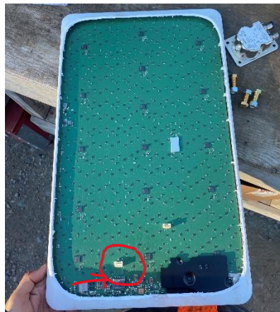
Figure 26, 27, 28, 29, Instructions for Cutting Starlink, Post Cut Starlink Dish
