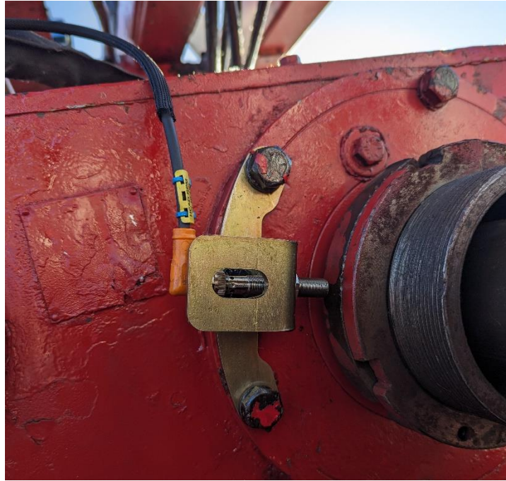
Figure 17 Head speed mounted on supplied bracket after being mounted.
